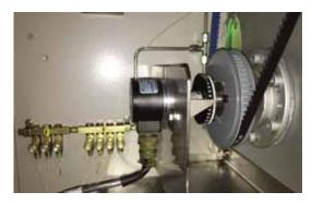
To check for a defective encoder, slowly hand-crank the machine while someone is watching the timing screen on the HMI operator display. The timing numbers should change by 1-degree increments. If the timing skips one or more numbers, the encoder is likely defective. Be sure to hand-crank the machine through a complete 360-degree rotation and verify that each timing number is displayed. A defective encoder can also increment backwards or jump a series of timing numbers.
