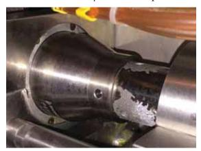
In the vast majority of installations, the nickel plating adheres for the life of the converter. However in some applications, the corrosiveness of the cleaning chemicals used may cause the nickel plating to peel off. This does not affect the operation of the converter. It will still successfully weld caps to the cartons. But there may be some concern about the appearance or about flakes of nickel coming off of the converter.
